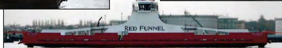
Red Kestrel in the Mersey on completion for Red Funnel, 2019 Capacity 12 HGV's and 12 passengers. 12.5 knots. Image Gordon Ditchfield
